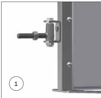
1 Distance between floor and lower edge of gate is 10 mm
