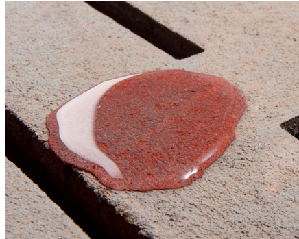
Treated slats with ACO Funki Protect - None water absorption.
