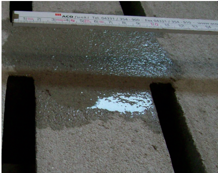
Untreated slats - Big water absorption.
