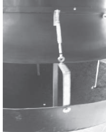
Fittings and stay tightener mounted on the light dimmer
