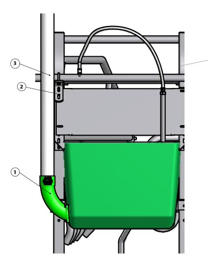
If there shall be casted with concrete around the integrated pipe (pos 1) and trough, then place a pipe (pos 3) in the angle and place a temporary brocket 5-10 mm (pos 2) to fix the brocket in the right position while the concrete is being casted.
