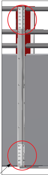
Mounting with connection screw from side.
