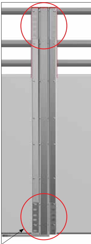
Mounting with connection screw from side.
