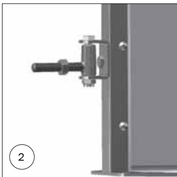
2 Distance between floor and lower edge of gate is 20 mm
