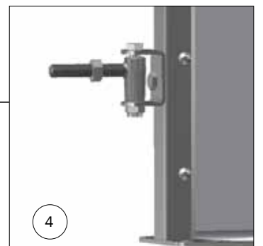
4 Distance between floor and lower edge of gate is 40 mm
