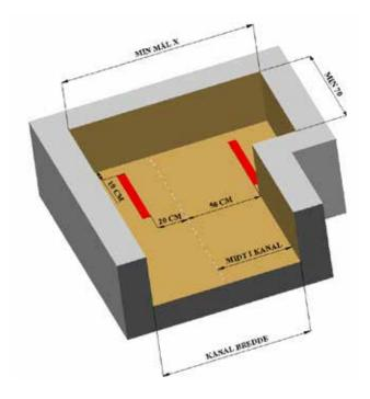
If channel is less then 90 cm, pit for drive unit should be at least 125 cm width.
