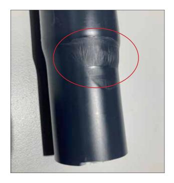
Avoid applying too much glue inside the pipe joint, as there will be a risk of etching the PVC.
