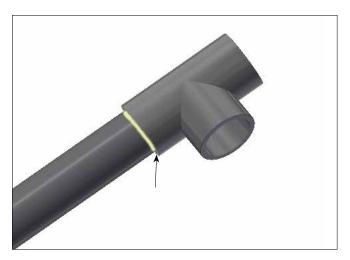
Remove excess glue. Leave to harden for 10 minutes
