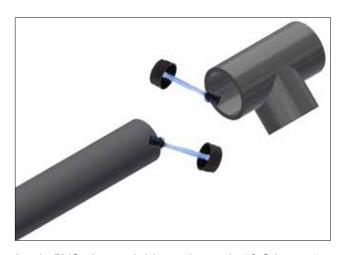
Apply PVC glue quickly and evenly (4-6 layers) on both adhesive surfaces (pipe thick layer, sleeve thin layer).
