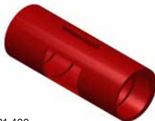
0221-400 VD2/VD6 CONNECTION FOR Ø50 MM CONVEYOR TUBE
