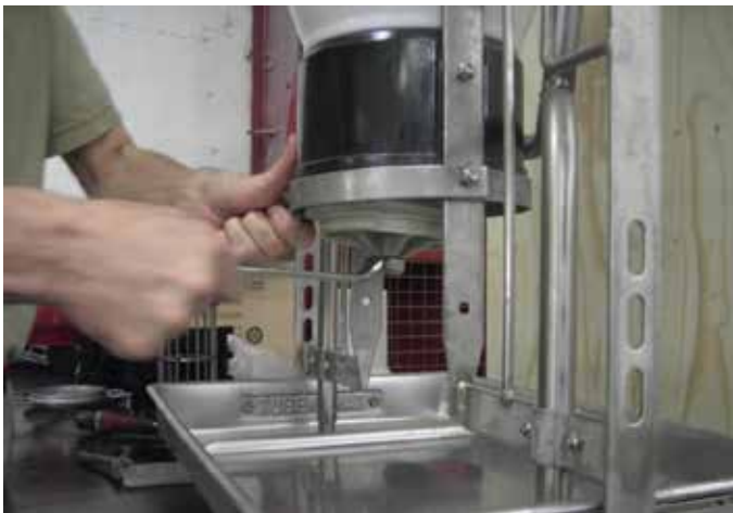
Remove 8 mm locking nut and screw feeding dispenser plate out (to the left).
