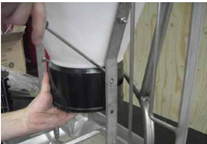
Remove 8 mm nut and push bolts in. Then, release the collar as it is shown, with the big flat screwdriver. As alternative solution - hit bolts out using hammer and punch.
