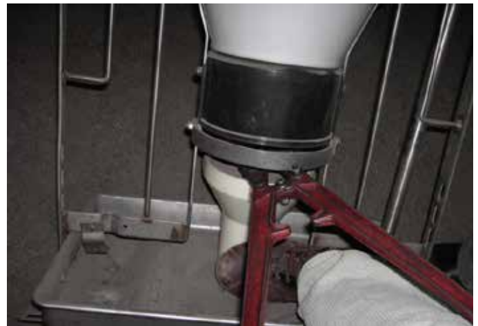
If it is not possible, release unit by cutting over adjustment bar with bolt cutter, as alternative use grinder.
