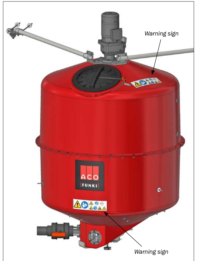
Where to place the warning signs
