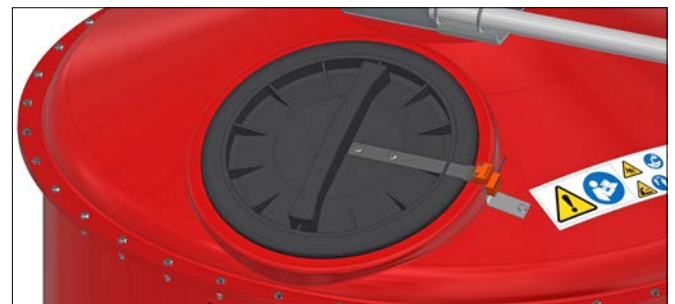
If the hatch is placed with the handle turned vertically, the safety switch bracket is mounted perpendicular to the handle of the hatch.
