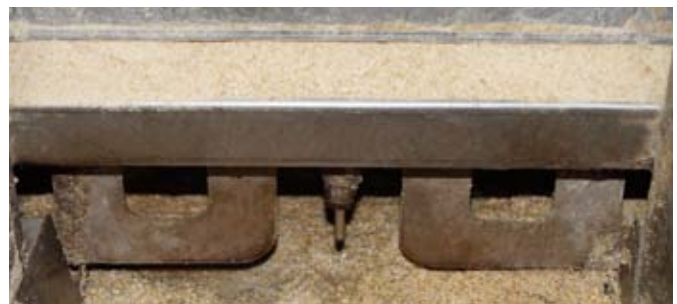
Water comes out of the press valves in the trough.
