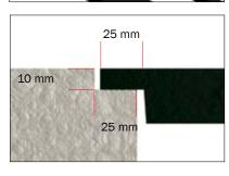
Cast iron slats have the same bearing surface and height as for ex. triangle slats, that can easily be replaced.
