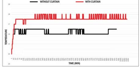
\*\*The test was made with an electrical heating plate. The temperature was measured each minute for at least 1000 samples. The diagram shows how the curtain improves the final temperature. The temperature data logger was placed in the same position, i.e. 100 mm from the floor and in the middle of the nest.
