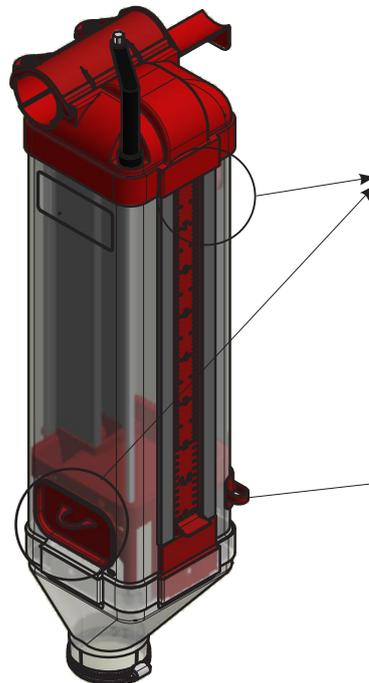
The release system is combined with a slide allowing adjustment of the feed amount even when having feed in the dispenser.
