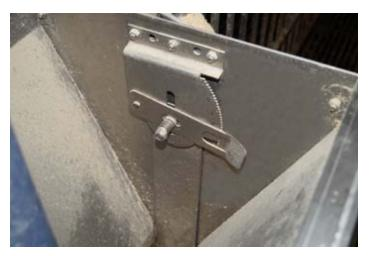
The adjustment system requires only two adjusters per feeder providing quick, accurate and consistent control of feed gate settings.
