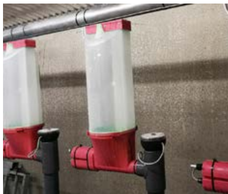
SCREW DOSING FOR FLOUR AND GRANULES WITH FLOW CONTROL SYSTEM
