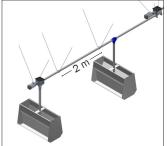
For better stability, we recommend to place the suspension chains every two meters.
