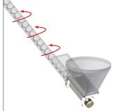
The auger coil must always run clockwise, seen from the inlet.
