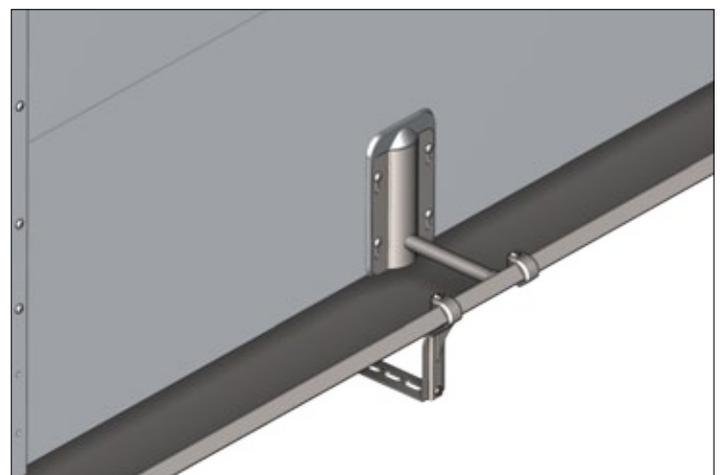
*For liquid feeding walls without integrated downpipes a rear plate for supporting legs is mounted*
