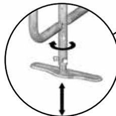
**Multi-adjustable foot** makes it easy to clean behind the stall and to adapt the stall to all types of floor.
