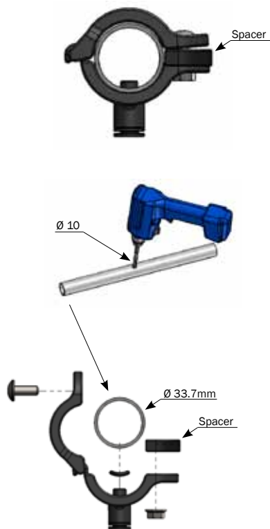
Mounting with master drill clamp (61195)
