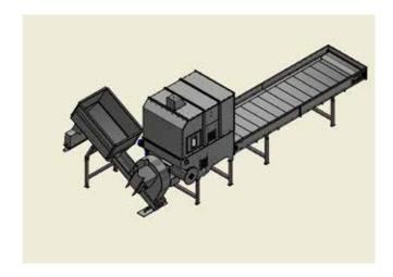
Automatic solution for big and round bales. There are built-in straw rivets, automatic tearing and filling. Here it is possible to use your own straw bales.
