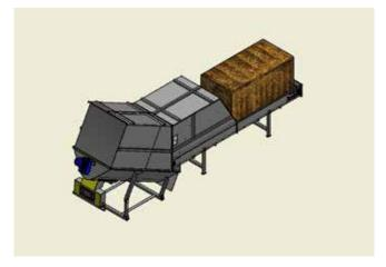
Automatic solution for prechopped big bales. It is well suited for filling with big bales, which are cut with a maximum length of 40 mm.
