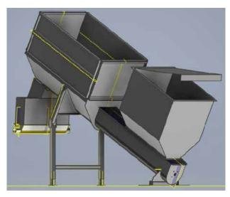
Solution with manual filling of container. It is simple and reliable. Suitable for filling with bedding, which is cut from external straw rivets and which can be purchased in sacks or loose.
